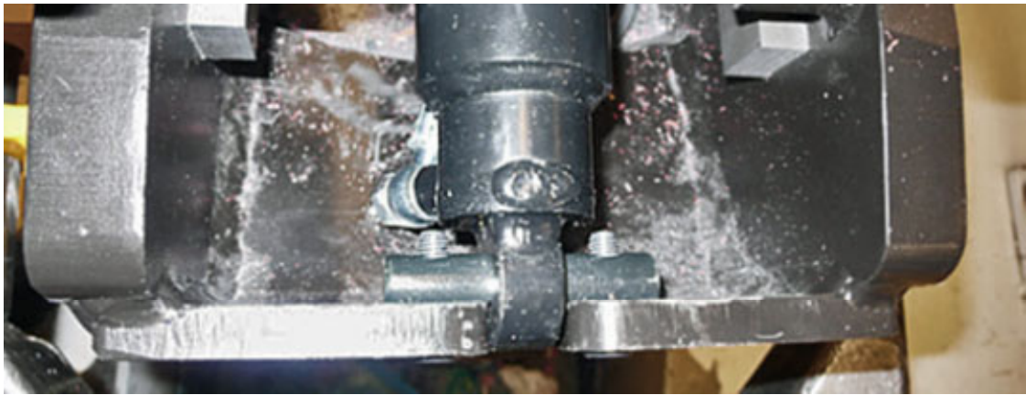
Hoses angled inwards to stay under cylinder
