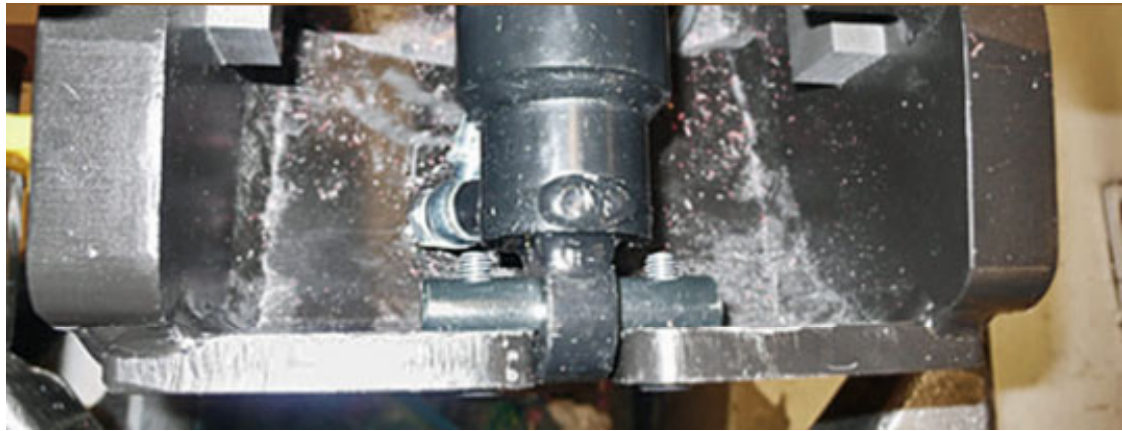
Hoses angled inwards to stay under cylinder
