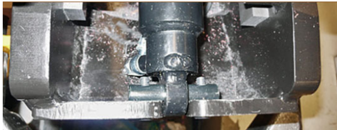
Hoses angled inwards to stay under cylinder
